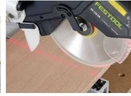
Dual line laser of the Kapex marks the exact width of the cut so the workpiece can be positioned from the left or right.
