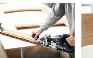
The corner and flat connector system enables stable connections that can be separated again at a material thickness of 30mm or higher in a 14mm connection.
