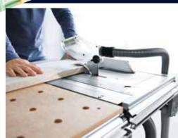
The V-groove around the outer edge of the MFT allows for the connection of the CMS system, as well as collection of available, sliding tables, mitre guides and stops.
