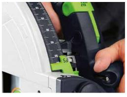
Easy to read and set: the dual cutting depth scale for work with and without the guide rail ensures precision every time.
