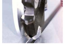
The feeler roller allows you to adjust the routing depth to suit the material thickness you are working with.
