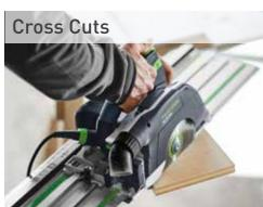
Attach the FSK cross-cutting guide rail to the HK Saws in seconds for fast, precise angle cuts.
