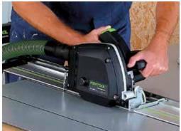
When paired with the Festool dustextraction and 36mm hose, faultless v-grooves are produced to professional standards without a trace of any ch
