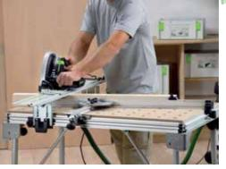
The guide rail adapter with hinge attaches the rail to the MFT table and slides effortlessly to produce perfectly straight cuts.
